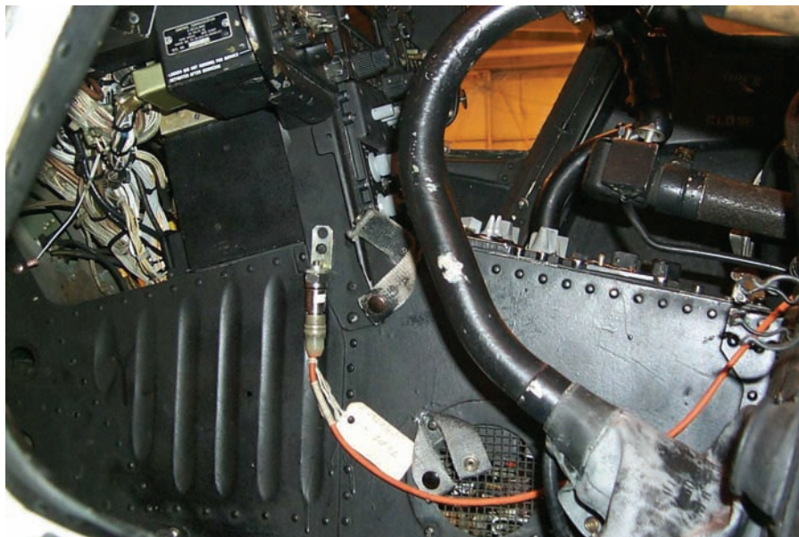
Figure 4. Vertical Accelerometer Installation
