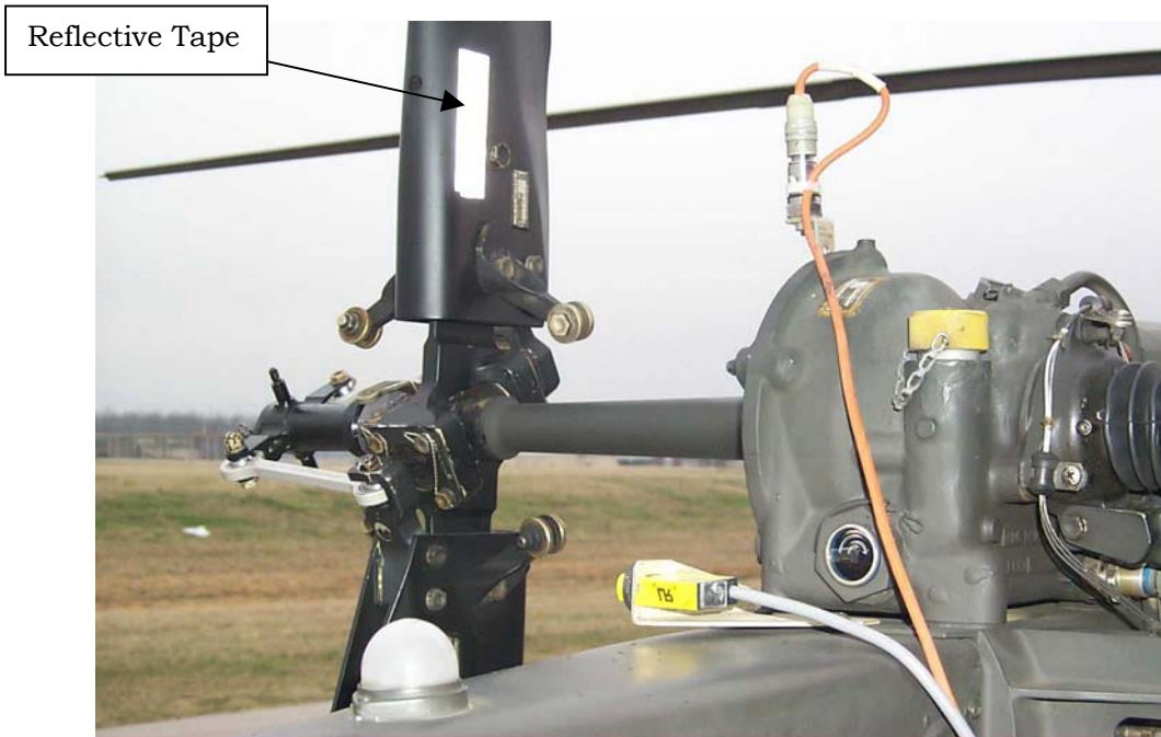
Figure 7. Reflective Tape Installation
