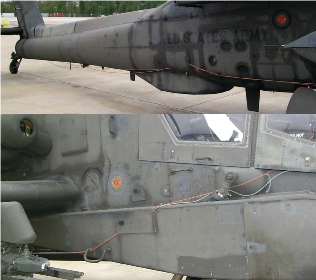
Figure 15. Tail Accelerometer Cable Routing
