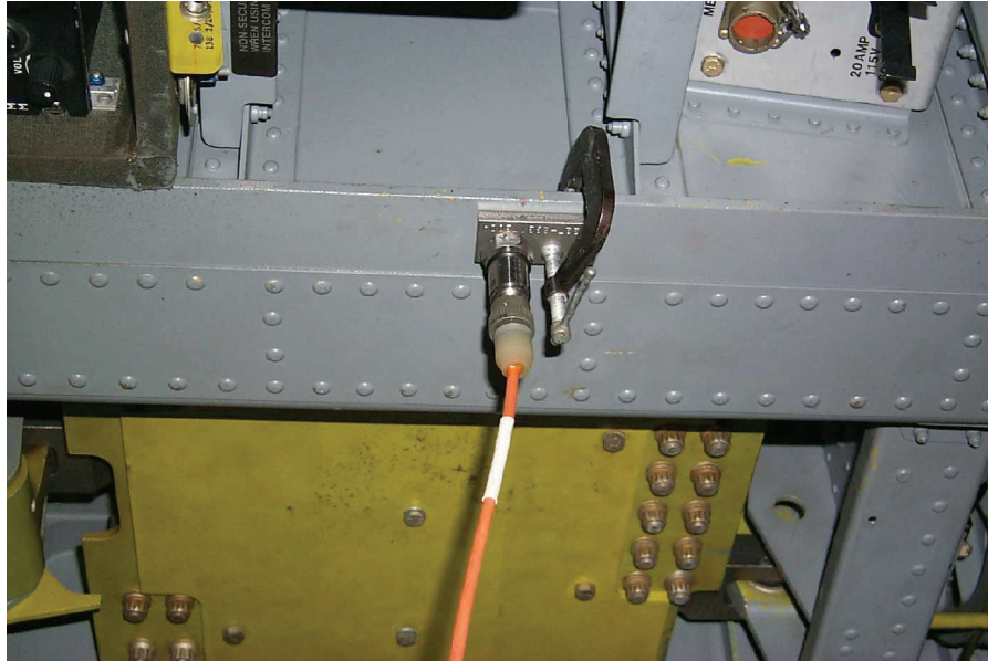
Figure 16. ABTUNE/BOXABS Tuning Accel. Installation (View looking up)
