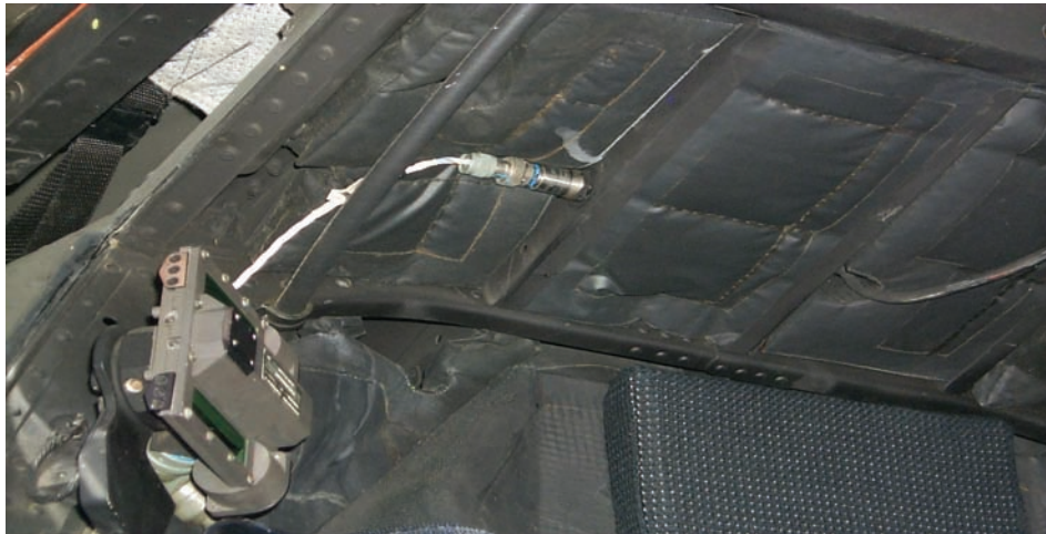
Figure 3. Lateral Accelerometer Installation (SPU/External Wiring)
